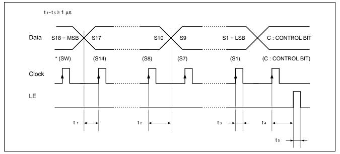
\* : Paranthesis data is used for setting divide ratio of programmable reference divider. On rising edge of clock shifts one bit of data in the shift register.
