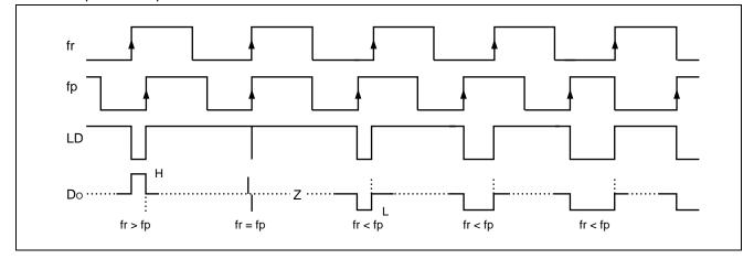
Phase comparator output waveforms are shown below.
